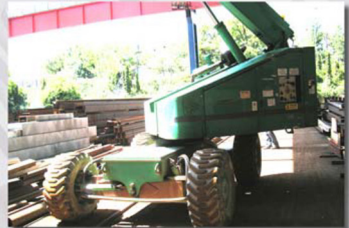
Manufacturer: T-REX 4WD Max Load: 400 kg Max Height: 22 m
