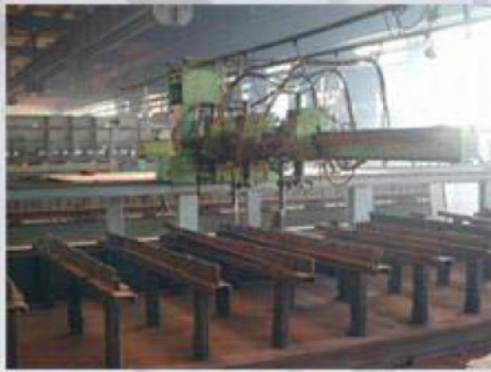
Name: Automatic gas cutting with photocell Type: CORTA Manufacturer: Messer Frankfurt-Germany Cutting area 3000x 18000 Max thickness 250 mm Average cutting speed: 34 cm/min Year of production 1981 Pieces: 1
