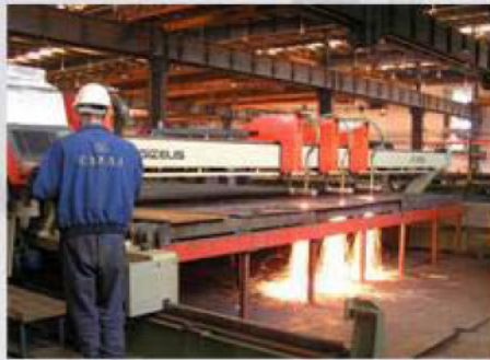
Name: Plasma cutting machine PANTOGRAPH Type: Fine focus 800 Manufacturer: Kjellberg Germany Max 180 mm average speed 200-1600 mm/ min Cutting area 24000x 6000 mm CNC Plasma and Oxygen cutting Year of production 2006 Pieces: 1
