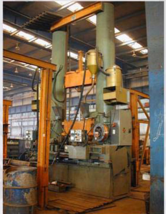
Name: Arc welding machine MASTER Type: ARMCO Manufacturer: ARMCO-Genova Italy Accessories: Aggregates (pcs=2) "IDEAL ARC" DC-1500 A, "The Lincoln Electric Company" -Cleveland, Ohio- USA, Steel profile dimensions: 700/200/3000 Year of production 1981 Pieces: 6
