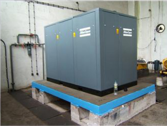
Name: Atlas - Copco Type: 4352 Manufacture: Atlas - Copco Capacity 25 m 3 /h Compressor 4352 Work pressure 9 atm. Year of production 2003 Number of compressors: 2
