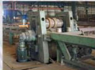
Name: Equipment for predeformation Type: IP 700x35 max; 150x10 min Manufacturer: Di Parmigiari-ItalyB max- 700 mm Max width Dmax – 35 mm Max thickness Leigh- no limit Speed: 14 m per min Year of production 1981 Pieces: 2
