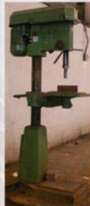
Name: Equipment for predeformation Type: Raddrizatrice 2000x30 Manufacturer: Di Parmigliari-Italy Max width 2000 mm Max thickness 30 mm Year of production 1981 Pieces: 1
