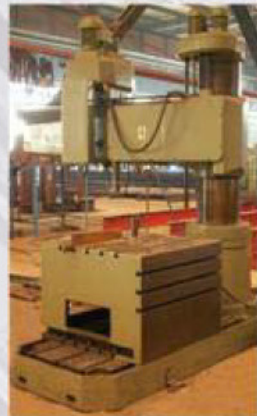
Name: Equipment for predeformation Type: Raddrizatrice 2000x30 Manufacturer: Di Parmigliari-Italy Max width 2000 mm Max thickness 30 mm Year of production 1981 Pieces: 1
