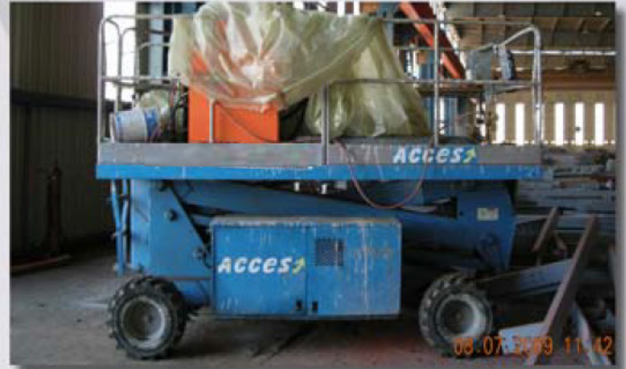
Manufacturer: UPRIGHT SL26SL DSL SCISSOR 4WD Max Load: 800 kg Max Height: 11 m
