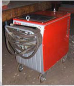
Name: JACKLE Type: Power Plasma Manufacturer: Germany Max:20A/88V-160A/144V Handy Plasma cutting machine Year of production 2007 Pieces 2
