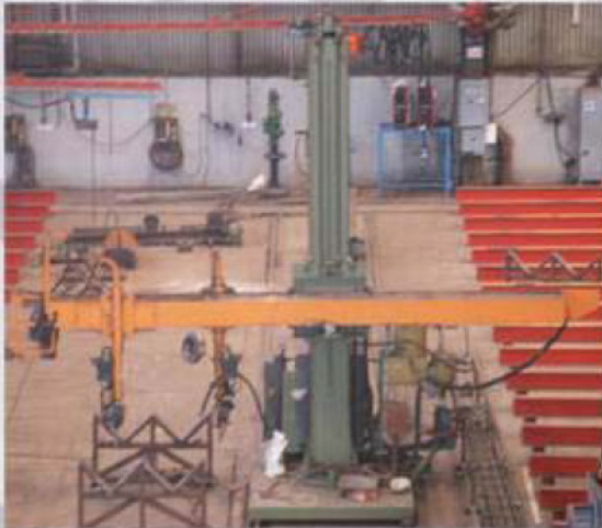
Name: Arc Welding Machine Type: MH 55/4 Manufactured: AMRCO-Genova Italy Accessories: Aggregates (pcs=2) "IDEAL ARC" DC=1500 A "The Lincoln Electric Company"-Cleveland, Ohio, USA Steel profile dimension: H/4200 - V/4500 Travelling: ??? = 60?? Height = 4,2 m Vertical = 4,3m Year of production 1981 Pieces: 2+1
