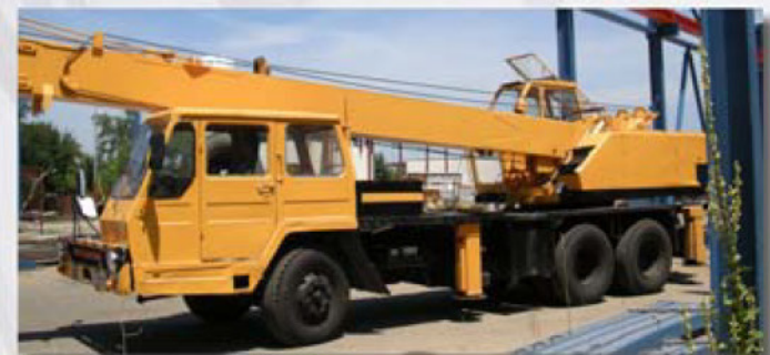
Manufacturer: KATO Max Load: 16 ton Max Height: 45 m
