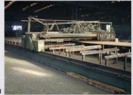
Name: Automatic gas cutting Type: SH - 5600 Manufacturer: Messer Frankfurt-Germany Max. number of burners: 8 pic. Min. distance between burners: 40 mm Max lenght: 26 m Max width: 4m Average cutting speed: 0,34m/min Year of production 1981 Pieces: 2
