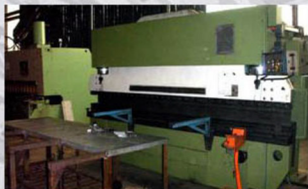
Name: BENDING MACHINE Type: Tip P1175 Manufacturer: TELEMÉQUANIQUE Max length 4050 mm Max thickness 18mm Year of production 1996 Pieces: 1
