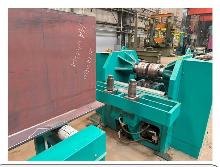
Type: Welded sections streightening
