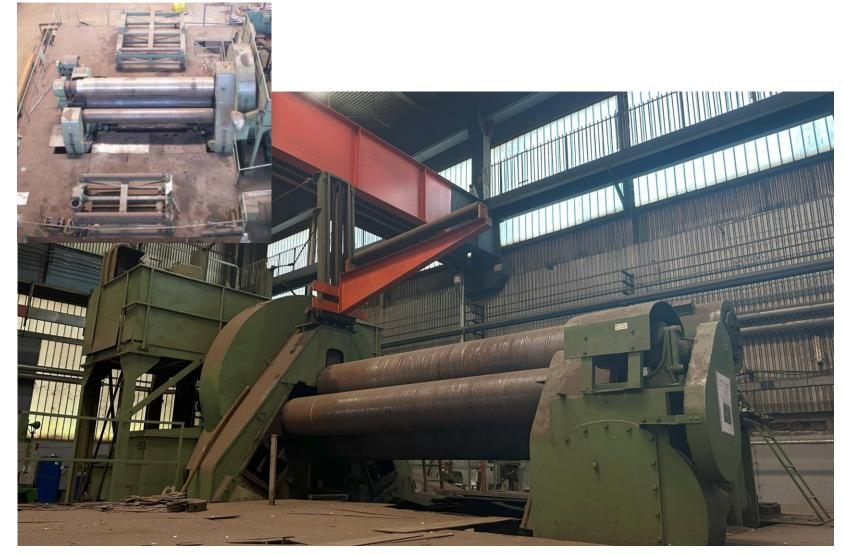
**Type:** Bending machine with conical bending device
