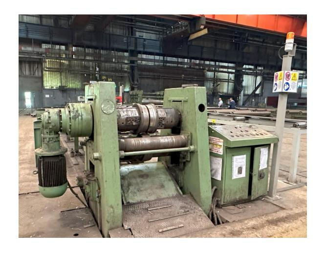
Type: Predeformation- plate straightening
